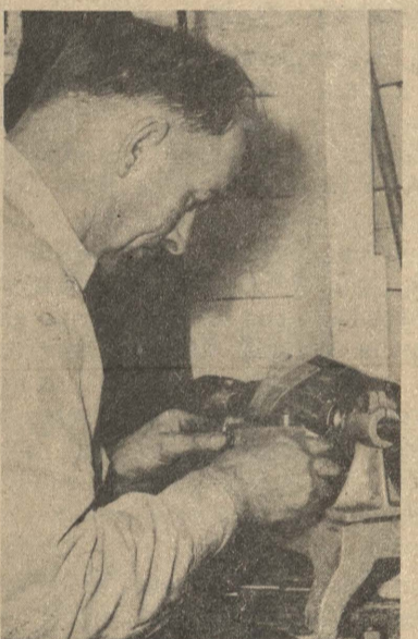
Fred Lofting, pipefitter days, Pipe Maintenance, reseats valve in shop.
