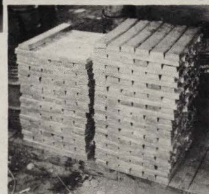
Thirteen thousand five hundred pounds of pig lead recovered from scrapped electrical cables. This pile is worth nearly $2,500.
