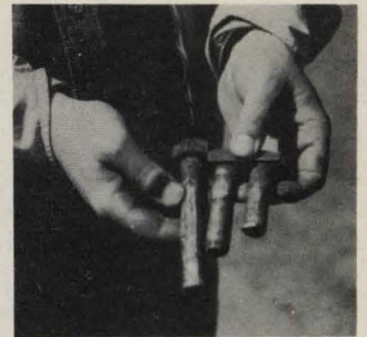
Driving bolts through "unfair" — out of line — plate holes damages threads, makes them useless. Some of them can be salvaged.
