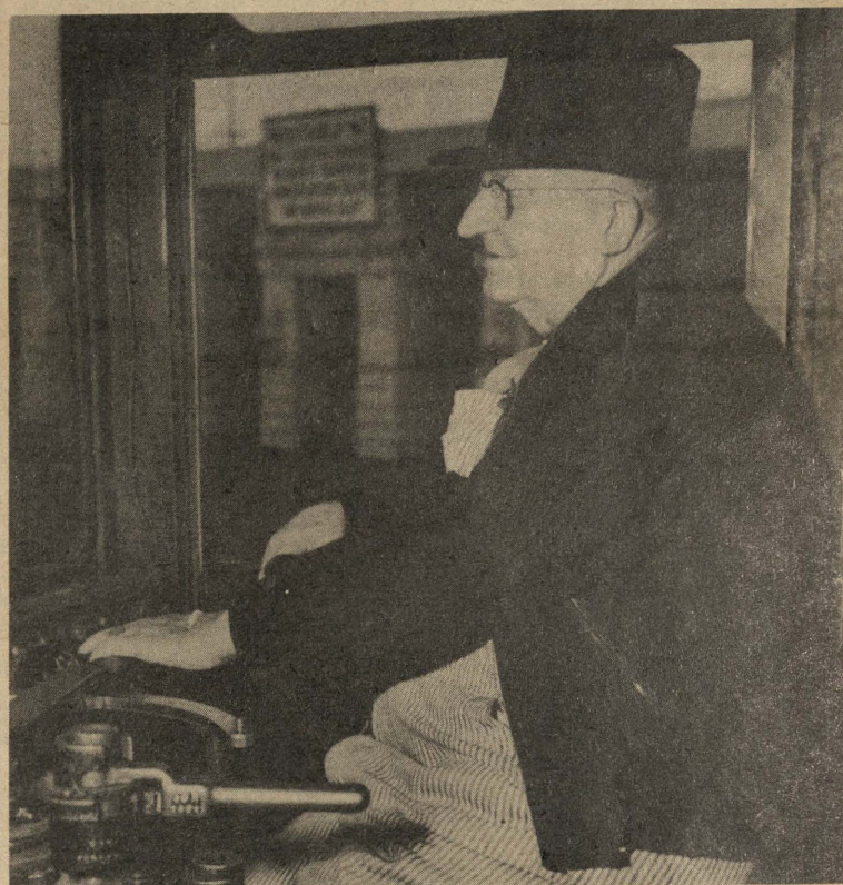
In true railroad style, Fred T. Ball, dinkey operator, sits in his cab with one arm on the window sill, the other hand on the throttle, watching the tracks ahead. By his left knee are the brake levers and the small brass lever that sets the bell on the cab to sounding its warning to workers.
