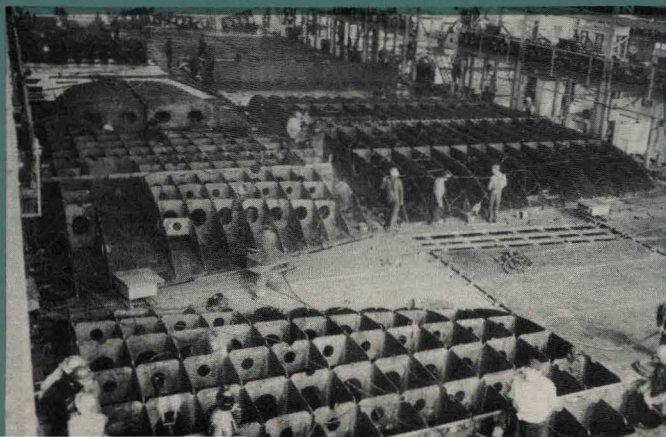
Huge inner bottom sections are prefabricated in an Assembly Shop bay.
