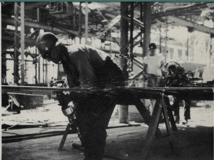
Making sure they'll fit. This man is grinding the edges of a plate in the Plate Shop.
