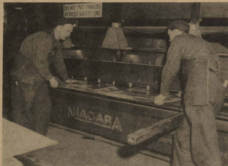
Mechanical Cutter Sheet metal workers use this 12-foot power shears machine to square and cut metal. Operating it are Les Hodel, left, and Bob Hedrick. (Oregon Ship photo)
