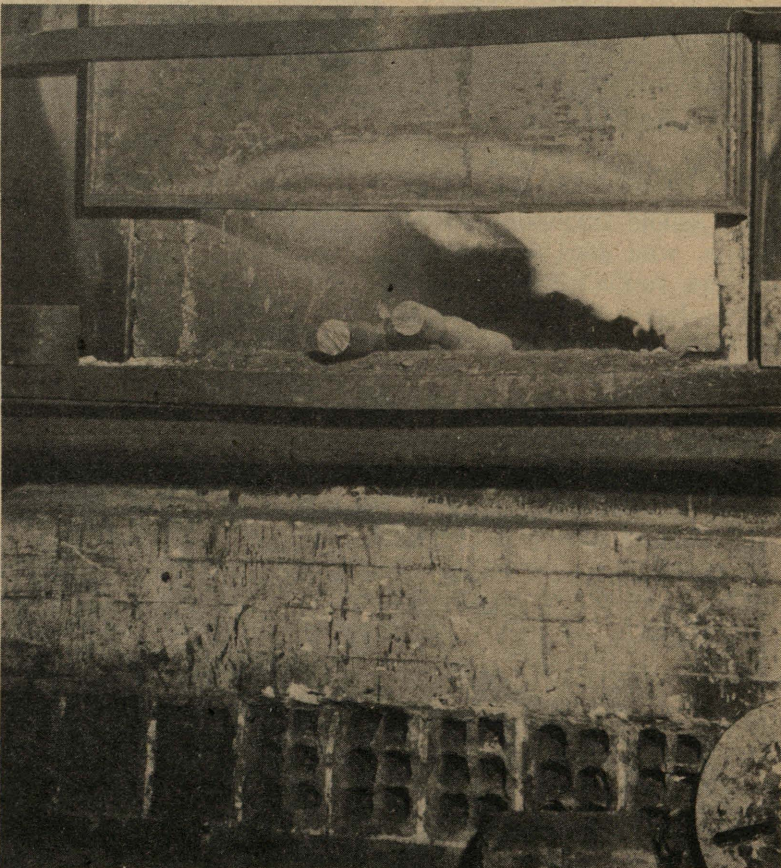
Here is the blast furnace where steel pieces are heated until they are ready to be hammered into shape. The furnace, heated by diesel oil under pressure, supplies the team of Jeffrey and Norgard with softened steel ready for the rapid tattoo of their heavy hammer.
