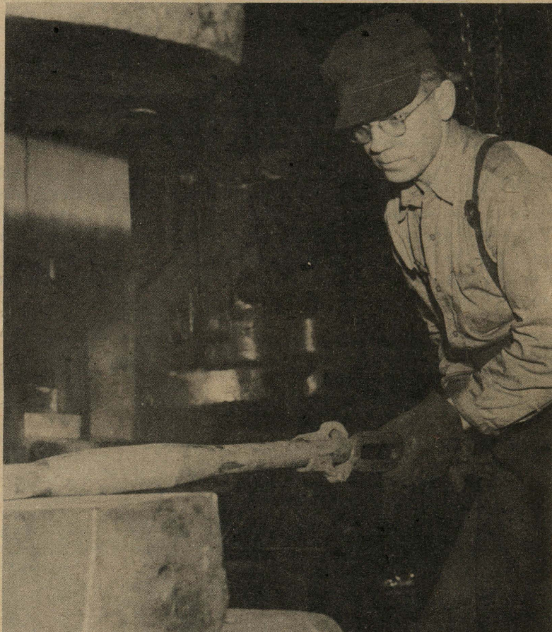
Holding a red-hot piece of steel on the bed of the heavy hammer, C. Norgard, heavy forger, watches the piece intently, turning and moving the future slab-dog so that the hammer blows strike in the precise spot needed for precise formation.
