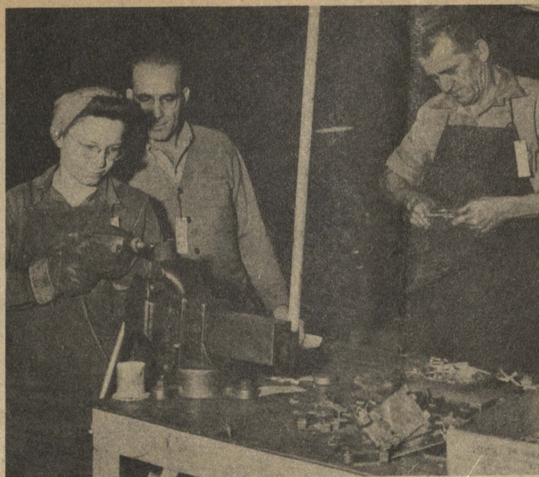
Almost half of employees in Electric shop are women. Here Olive Street operates a one-quarter inch tap gun on terminal block base while Leadman Floyd Englet looks on. At right, C. R. Gill prepares hangers.
