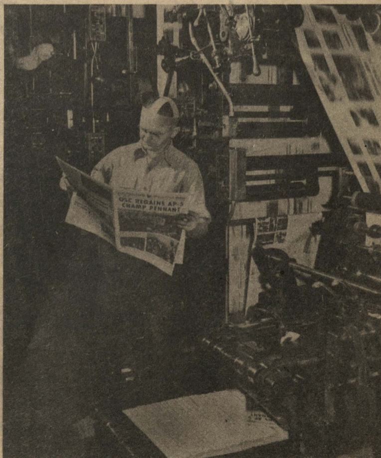
The Whistle Is Printed The above web-fed offset press, located in the Daily Journal of Commerce at S.W. 14th and Morrison, Portland, can shoot out Bosn's Whistles at the rate of 12,000 an hour. There is only one other like it on the Pacific coast and only a few others in the nation. Pressman John Meyer, above, studies ink distribution on the first few copies. Story, page 7.
