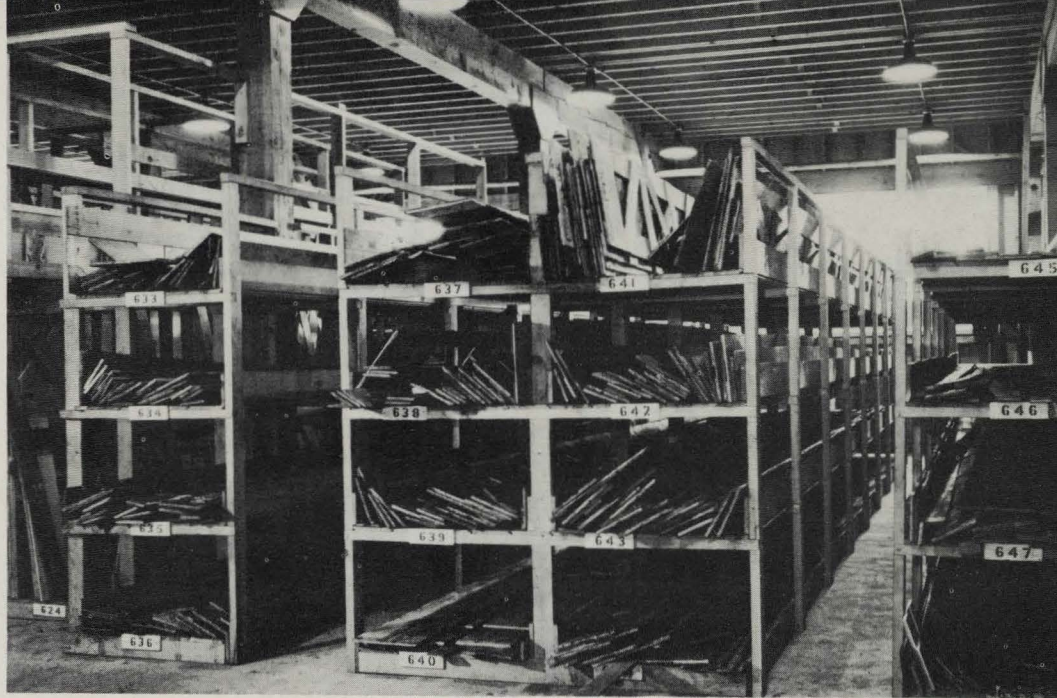
Templates are stored according to size—note bin numbers. Duplicates are stenciled on each mold.
