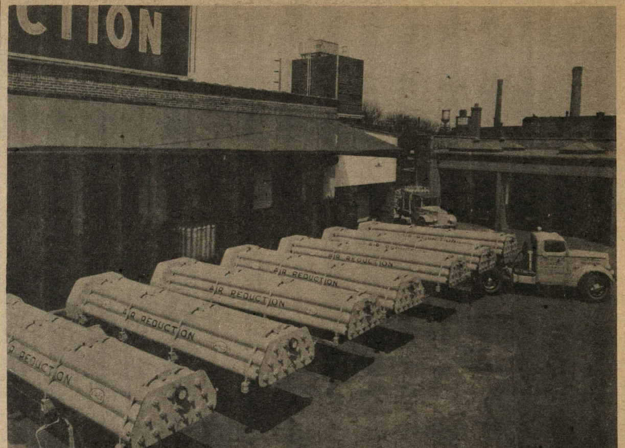
Oxygen is transported in huge trailers carrying cylinders, such as are shown above. Each cylinder contains 244 cu. ft. of compressed gas at a pressure of 2200 lbs. per square inch.
